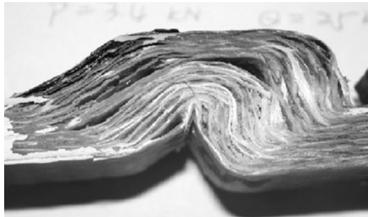
Figure 9. The failed fiberglass reinforced composite column exposed to the fire heat flux Q = 25 \text{ kW/m}^2 under the constant axial compressive load, P , corresponding to a stress of 10.5 \text{ MPa} (based on the original section).
