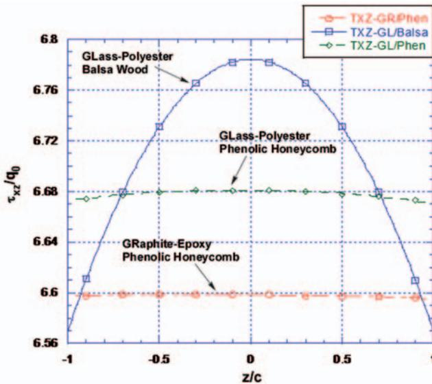
**Figure 5.** Through-thickness distribution in the core of the transverse shear stress,  $\tau_{xz}$ , at  $x = a/10$ , for three face/core material combinations.
