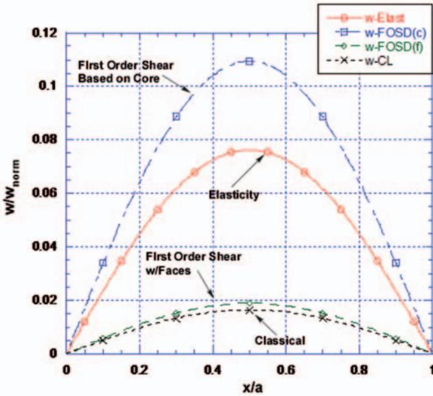
**Figure 2.** Transverse displacement,  $w$ , at the top,  $z = c + f$ , for the case of graphite/epoxy faces and glass phenolic honeycomb core.
