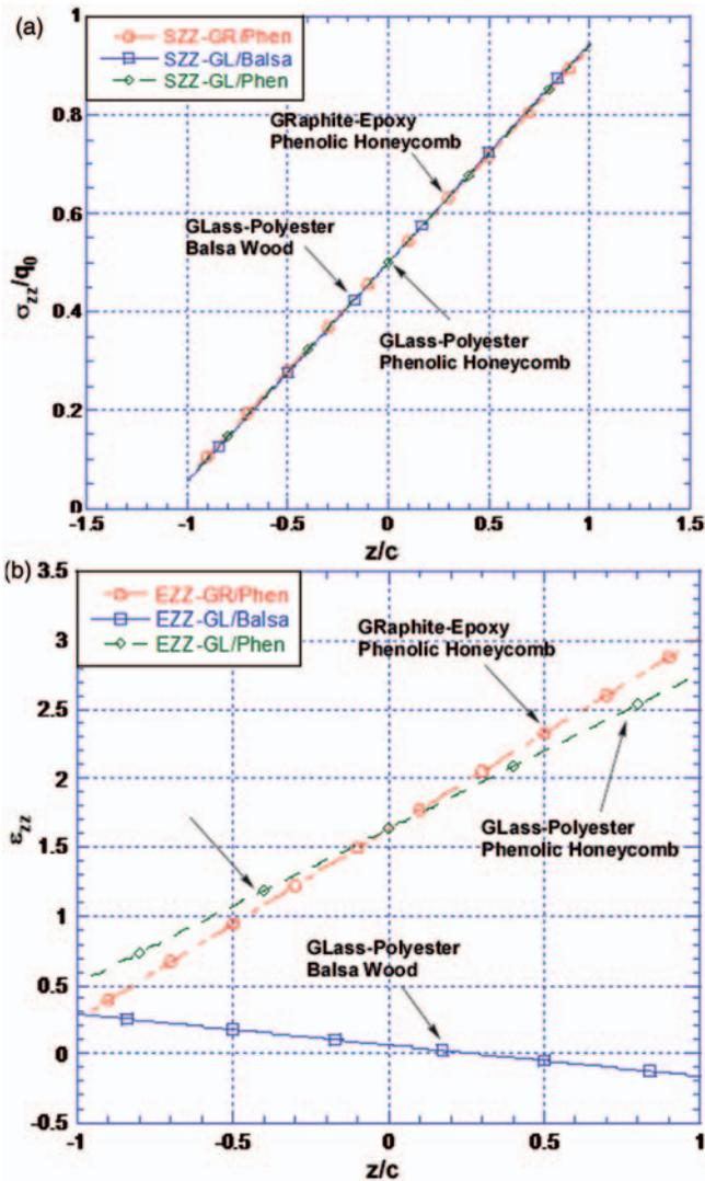
**Figure 4.** Through-thickness distribution in the core of the transverse normal stress (a)  $\sigma_{zz}$ , at  $x = a/2$ , for three face/core material combinations. (b) transverse normal strain,  $\epsilon_{zz}$ , at  $x = a/2$ , for three face/core material combinations.
