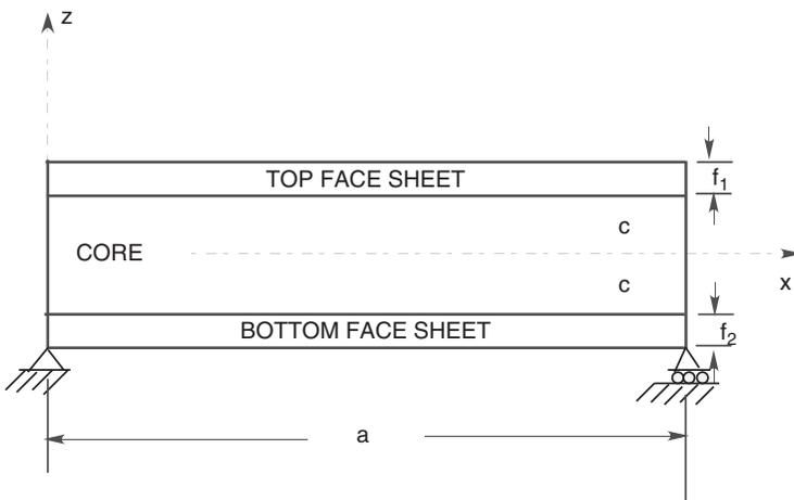
**Figure 1.** Definition of the geometry and coordinate system for the sandwich beam.
