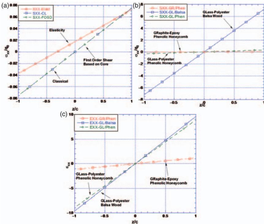
**Figure 3.** Through-thickness distribution in the core of; (a) the axial stress,  $\sigma_{xx}$ , at  $x = a/2$  for; (a) the case of graphite/epoxy faces and glass phenolic honeycomb core, (b) axial stress,  $\epsilon_{xx}$ , at  $x = a/2$  for three face/core material combination, and (c) the axial strain,  $\epsilon_{xx}$ , at  $x = a/2$ , for three face/core material combinations.
