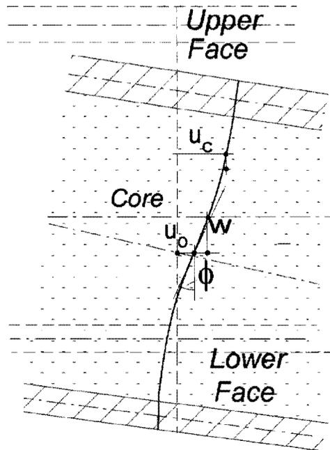
**Figure 3.** Displacement pattern of the HOSDT model through depth of panel.
