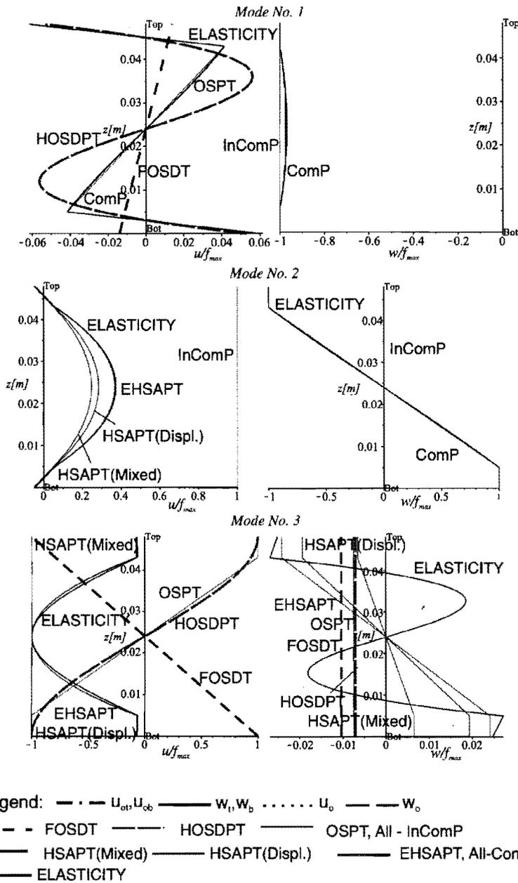
**Figure 6.** Three eigenmodes of stresses of the first half-wave number through depth of panel for various computational models and the elasticity solution. FOSDT: first-order shear deformable theory; HOSDPT: high-order shear deformable theory; OSPT: ordinary sandwich panel theory; HSAPT: high-order sandwich panel theory; EHSAPT: extended high-order sandwich panel theory.
