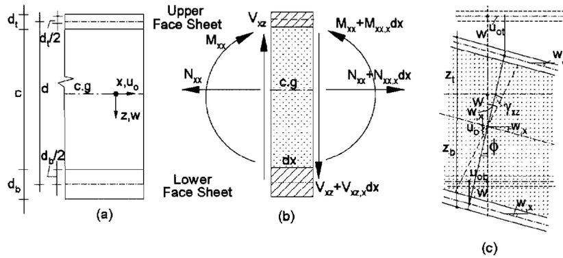
**Figure 2.** FOSDT displacement pattern through depth of panel. FOSDT: first-order shear deformable theory.
