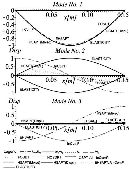
**Figure 5.** Three eigenmodes of displacements of the first half-wave number along panel for various computational models and the elasticity solution.
