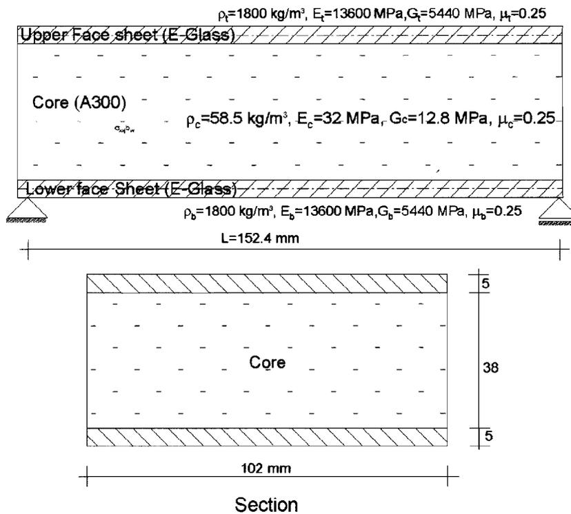
Figure 4. Layout of a sandwich panel and a typical section [17].
