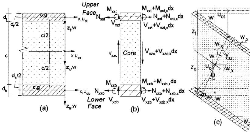
**Figure 1.** Coordinate system, stress resultants and displacement pattern for the OSPT model: (a) coordinate system; (b) stress resultants; (c) zig-zag displacement pattern. OSPT: ordinary sandwich panel theory.
