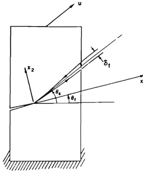
Fig. 2. *J*-integral parameters.
