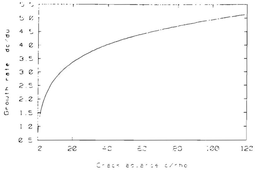
Fig. 4. Quasi-steady crack growth rate vs. crack advance.
