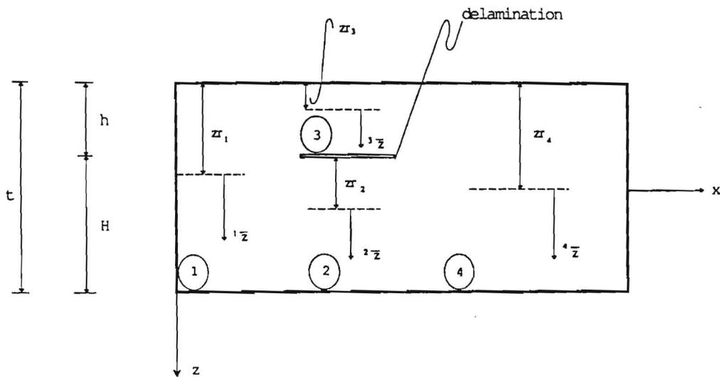
Fig. 4. Geometry and sign convention.
