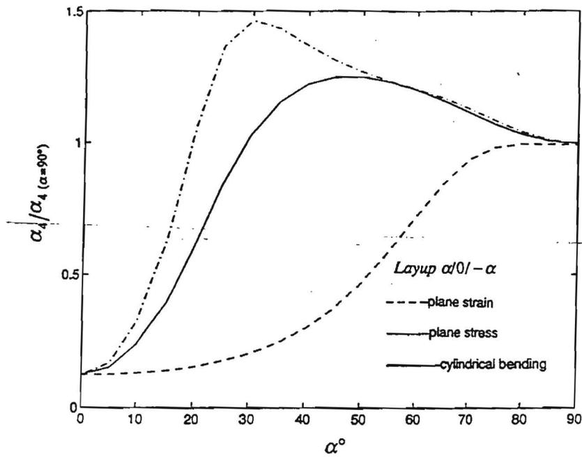
Fig. 3. Bending moment coefficient  $\alpha_4$  vs fiber orientation  $\alpha$  for the  $\alpha/0/-\alpha$  layup.
