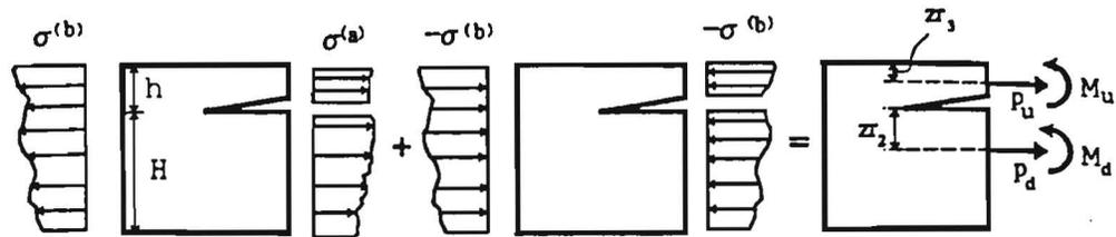
Fig. 5. Stress superposition scheme.
