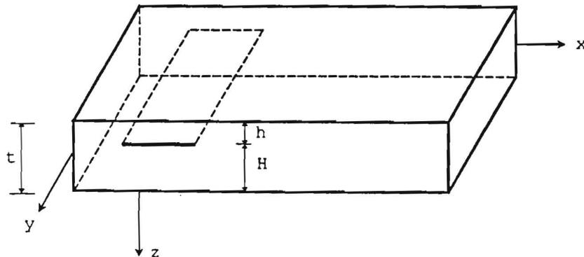
Fig. 1. Laminate with a delamination through the width.
