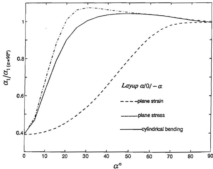
Fig. 2. Axial force coefficient  $\alpha_1$  vs fiber orientation  $\alpha$  for the  $\alpha/0/-\alpha$  layup.
