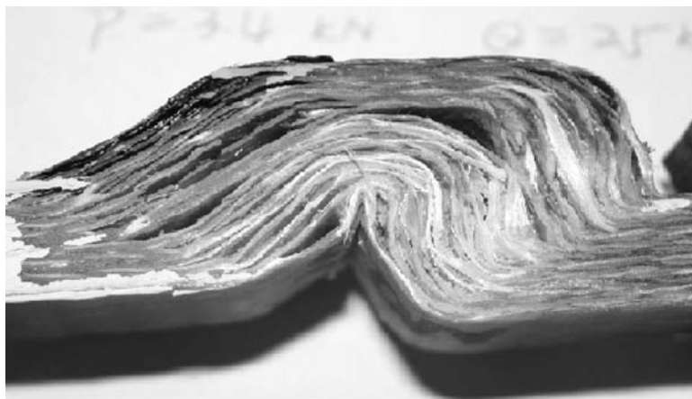
Figure 10. The failed fiberglass reinforced composite column exposed to the fire heat flux Q = 25 \text{ kW/m}^2 under the constant axial compressive load, P , corresponding to a stress of 10.5 \text{ MPa} (the stress is calculated based on the original section geometry).
