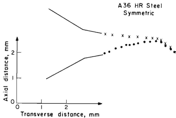
Fig. 10b. Fracture surface profile for the A36 hot rolled steel symmetric specimens.
